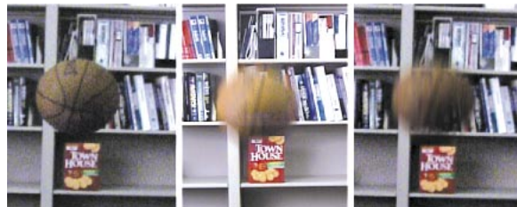
Figure 10: A dropping basketball was filmed with two cameras. The left image was shot with a shutter speed of 0.001 seconds, while the center image is from a camera with a 0.017 seconds shutter. We processed the crisper sequence to render the image on the right, simulating the the longer exposure. As expected, the blur has been mimicked and the original lighting is retained.
